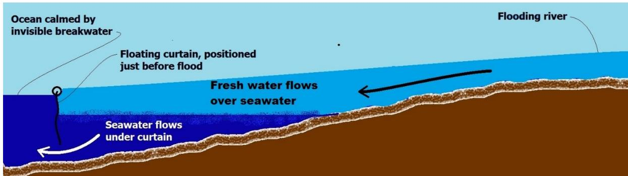
Fig. 4 – Elevation section of floating curtain during a flood
