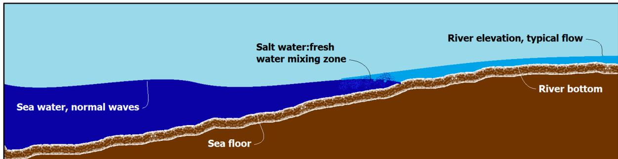
Fig. 2 – Elevation longitudinal section of river flowing into the sea
