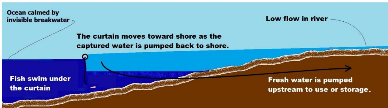
Fig. 5 – Elevation section of floating curtain contracting during fresh water storage
